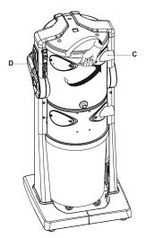
After exchanging their housings, reassemble the intake of the "C" exhaust pipe and the "D" closing sheet by fastening the screws. Now rotate by 180° the intake of the exhaust pipe as shown in the picture.
