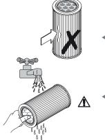
Check the filter surface is not cut. If this is the case, the cartridge should not be used again.
