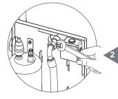
Screw the suction socket on the suction plug; check it has been firmly tightened. Close the cover made of thermoformed material.
